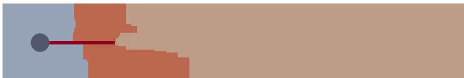
Figure 2. Split configuration using four subdomains. Load balancing issues are obvious.
